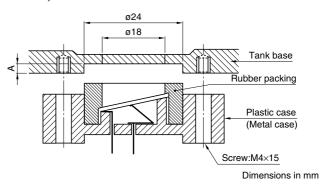
The transducer can beak off if the A dimension depth is shallow. TDK recommends a 2mm A-dimension depth and a screw tightening torque of  $0.6N \, \bullet \, m$ .
